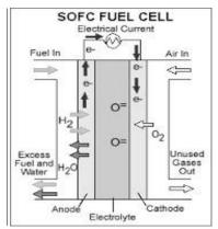
Operating temperatures of these cells are (800-1000 degree centigrade).they run on a variety of fuels including natural gas.
