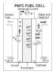
The porous electrodes used in PAFC's contain a mixture of the electro catalyst supported on carbon black and a polymeric binder to bind the carbon black particles together forming an integral structure. A porous carbon paper substrate acts as a strong support for the electro catalyst layer and as the current collector.
