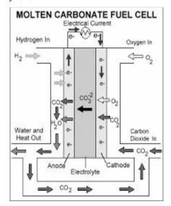
These ions combine with hydrogen to form water on the cathode side. During the reaction co2 and electrons are released.
